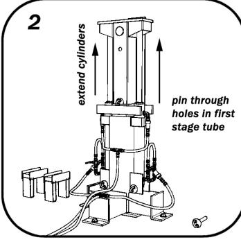
Raise first stage with hydraulic ram. Hold in position with pin through holes in first stage tube.
