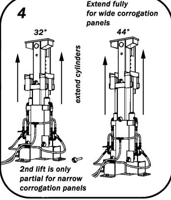
Raise 2nd stage with hydraulic ram. Hold in position with pin through holes in 2nd stage tube (optional)
