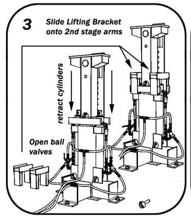
Open ball valves, retract cylinder. Close Ball valves in preperation for next lift. Place lifting brackets on second stage arms.
