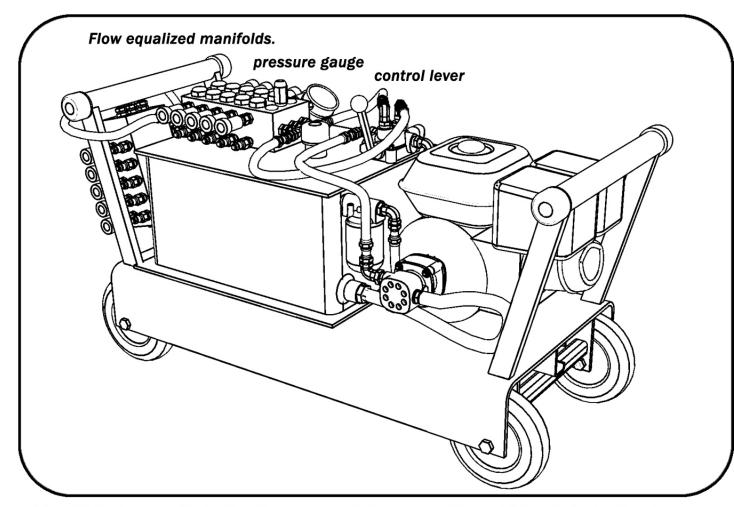
The 20 jack capacity hydraulic power unit is powered by a 13 hp 4 stroke Honda Engine. This power unit uses manifolds with integrated flow equalizers to keep the bin level automatically. The manifold is set to provide an equal flow of 1/2 gpm to each jack.
