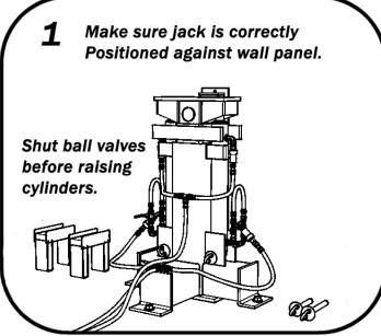
Place jack in position. Secure Jack to Concrete Hook up hydraulic lines. Shut ball valves before lifting. Lifting brackets not used for first lift.
